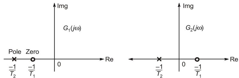
⇒ The *minimum phase function* has unique relationship between its phase and magnitude curves. Typical phase angle characteristics are shown below:
